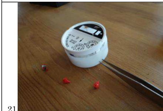
Remove the lid to push part of the hook
