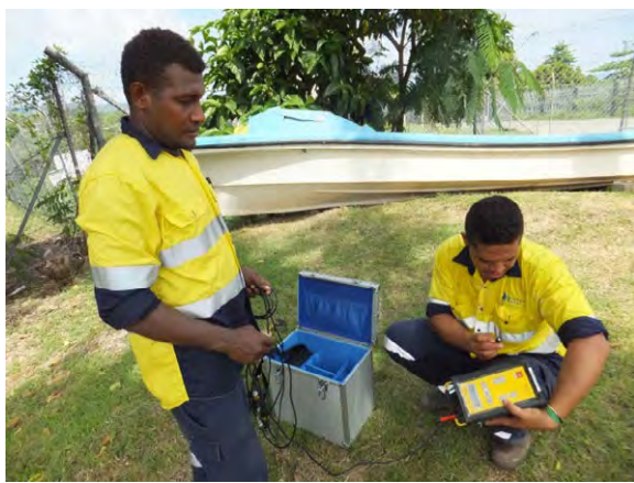
Figure 6.4-3 Identifying Leak Points by a Leak Noise Correlator
