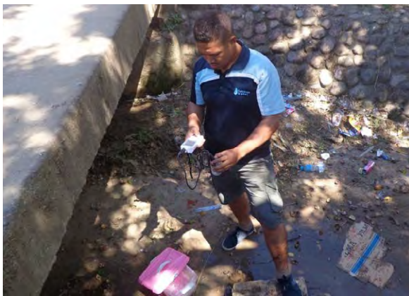
Figure 6.4-1 Surface Water measured by using Residual Chlorine Tester
