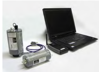
Figure 2-1 Water Pressure Logger
