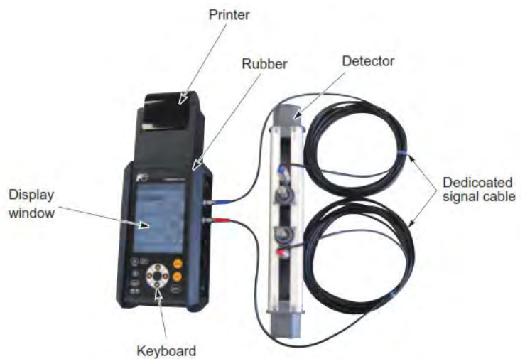
Figure 1-2 Components of Ultrasonic Flow Meter
