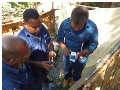
Figure 4-13 Residual Chlorine Meter
