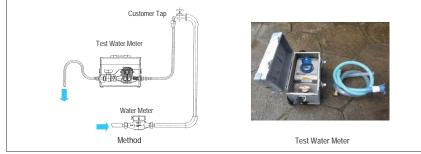
Figure 3-11 Method of Checking Accuracy of Test Water Meters
