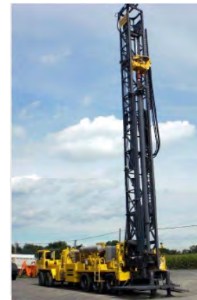
1. Rotary table-type Truck-mounted rig Source: http://www.esmap.org/sites/esmap.org/files/Bailey_Exploration(Day1)_0.pdf
