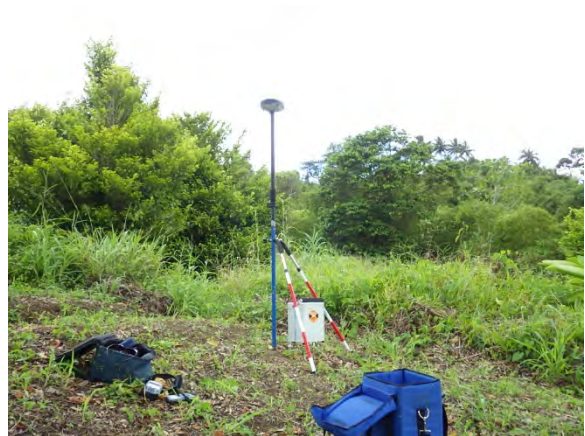
Gravity Survey (Gravimeter and GPS)
