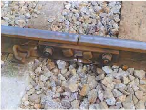
Measuring fishplate's stress
