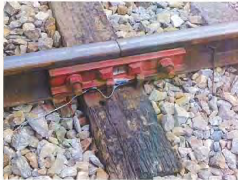
Measuring fishplate's stress
