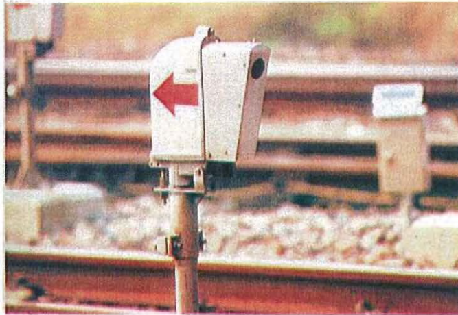
Photo 40.9 Example of crossing obstruction detection device
