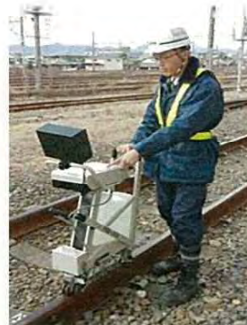
Photo3.5.2. Staff is inspecting the rail by ultrasonic rail flow detector
