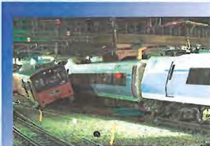
Train collision due to shunting signal violation (JR Chuo Line in 1997)
