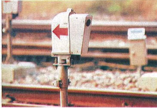
Photo 40.9 Example of crossing obstruction detection device
