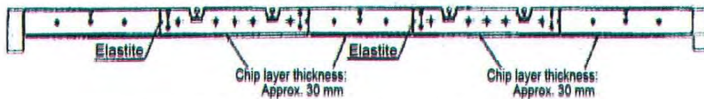
Photo 40.6 Example of continuous concrete block track crossing
