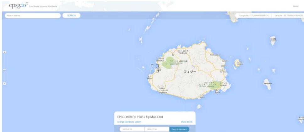
Figure 10-11 Software for the Conversion between the Latitude/Longitude and FMG Coordinates
