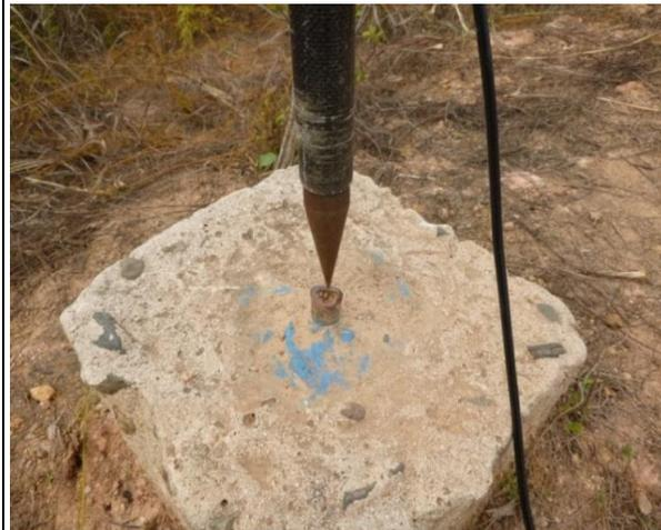
Each of the two national control points, SS11233 and SS3506, was surveyed using RTK-GPS (Table 10-5). The errors in this GPS surveying were proven to be below the allowable limits.
