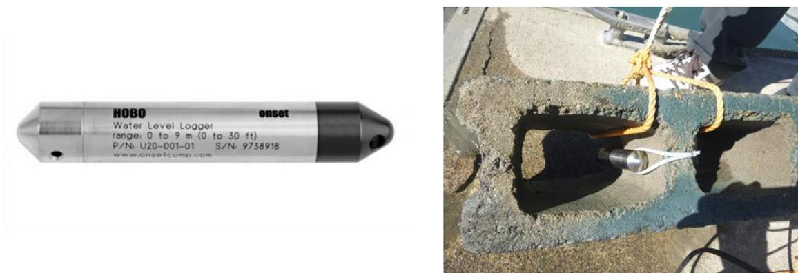
Figure 10-20 Pressure-sensor Water Gauge, U20 Water Level Logger, (left) and Gauge Tied to Concrete Block before Installation (right)
