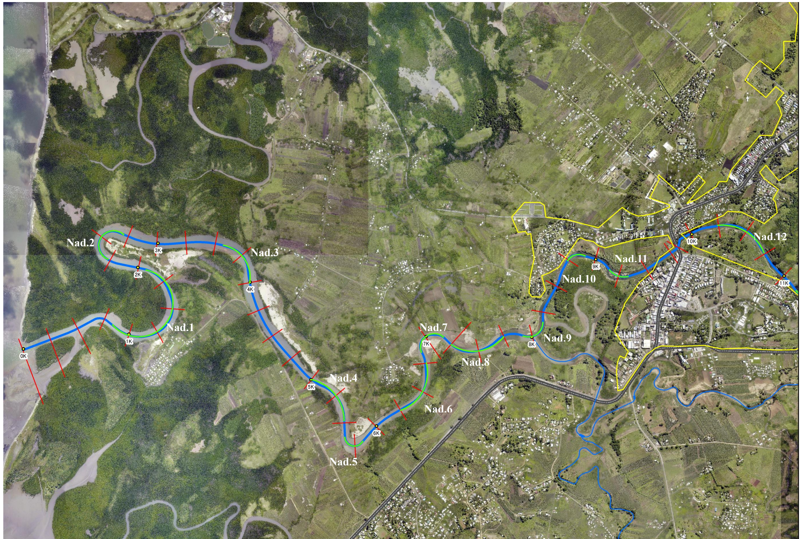
Figure8-6 Location of Bend Sections for Smoothing (Nadi River, Section from Nad.1- Nad.11)
