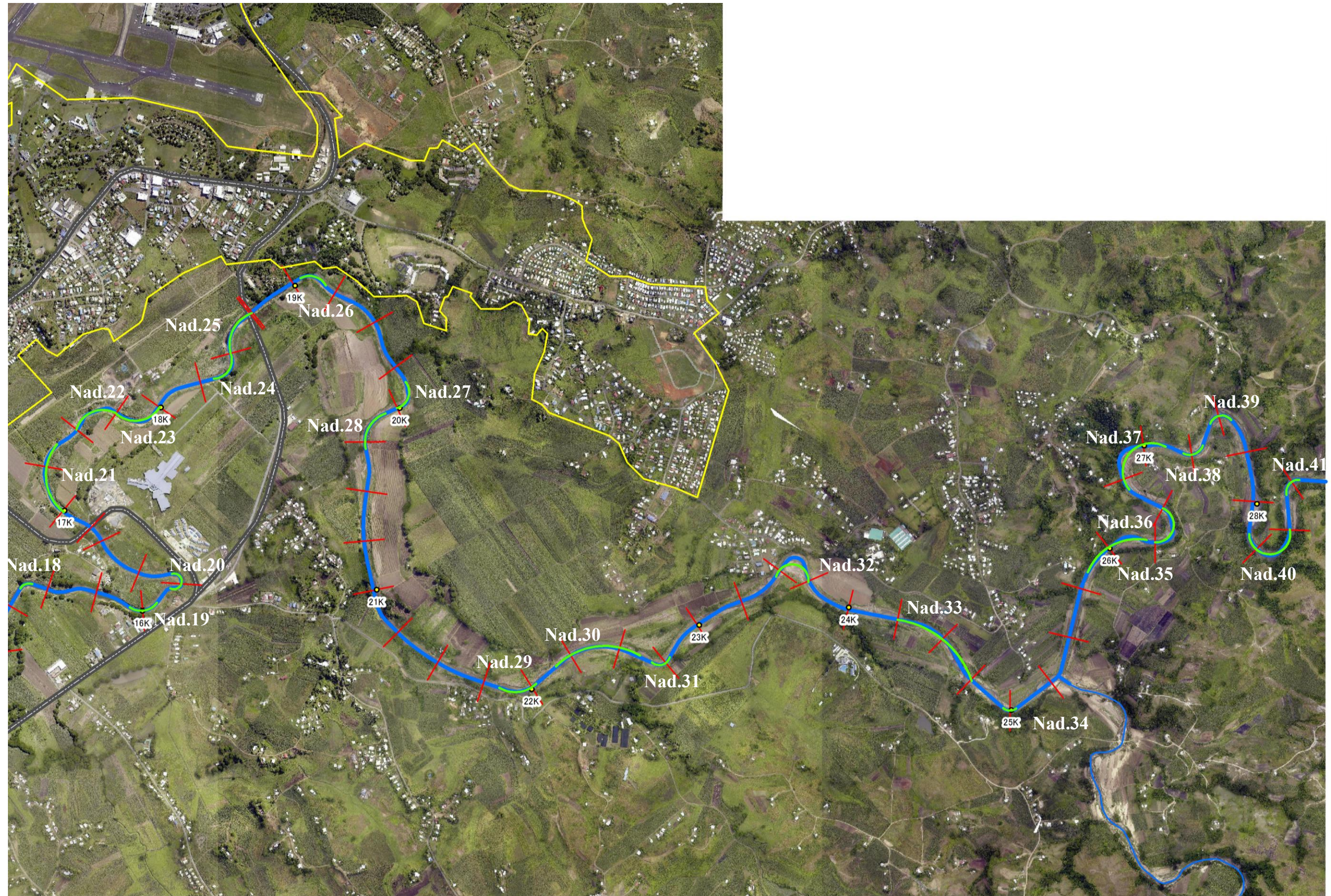
Figure8-8 Location of Bend Section for Smoothing(Nadi River, Section from Nad.28- Nad.41)
