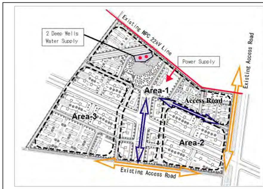
Figure 6-11 Construction Division Plan
