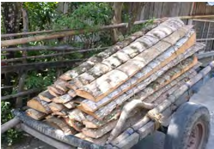
Photo 1-13: Coconut slabs for pillar
