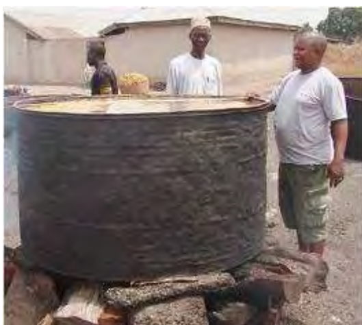
Figure 2-1-5: Large drum for soaking and steaming used by the Lafia Millers and Dealers Association in Nasarawa State
