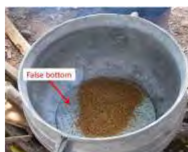
Figure 2-1-9: False bottom in the traditional cooking pot
