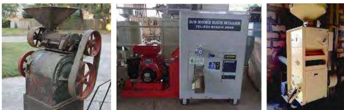
Figure 2-1-14: Stand-alone type small-scale milling machines available in Nigeria. From left, Engelberg steel huller (Made in India or China), friction-type milling machine (South Korea), and one-pass milling machine (Indonesia)
