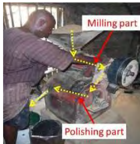
Figure 2-1-15: Passing twice in the milling chamber and once in the polishing compartment
