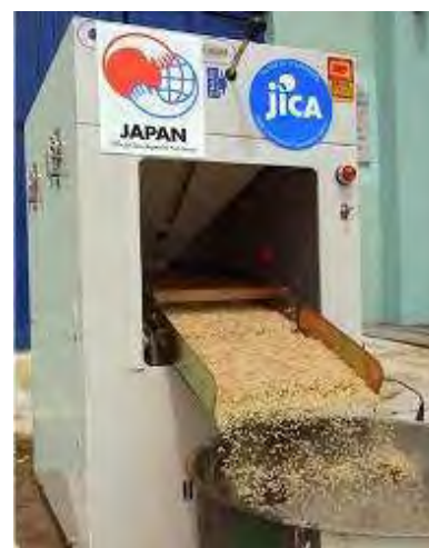
Figure 2-1-16: Small de-stoner made in South Korea, available in Nigeria
