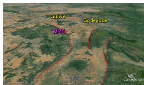
F: Site MZ5 Located in the Small Rift Valley (Red Line: Presumed Fault)
