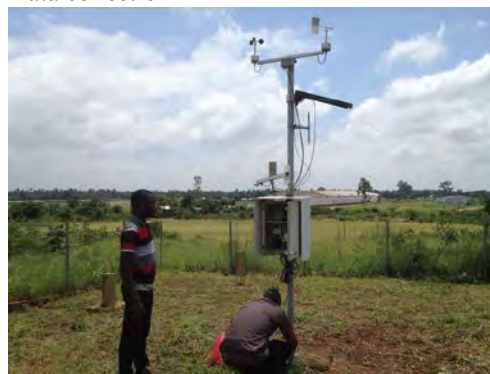
Automatic weather station with a solar panel and a control panel
