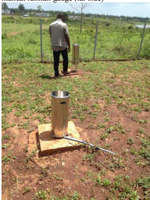
Automatic rainfall gauge (near side) and manual rainfall gauge (far side)
