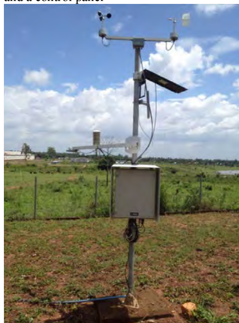
Automatic weather station with a solar panel and a control panel
