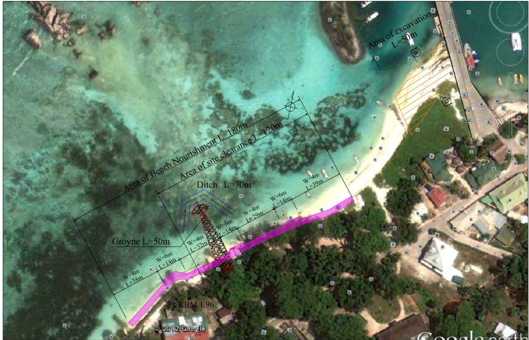
Figure 6-2-4: Groyne and Nourishment Plan at La Passe
