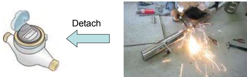
Figure 4.5 Treatment of Meter with high temperature of the welding
