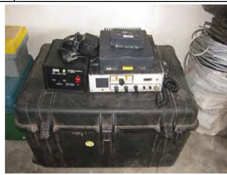
Photo-20 Workable wireless equipment (HF/VHF)
