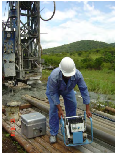
1.Measuring of the water level before Logging
