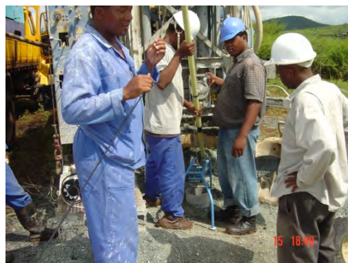
10. Inserting the probe into borehole
