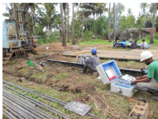
12. Carrying out the borehole logging
