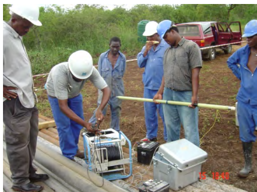
9. Connecting the probe to the winch
