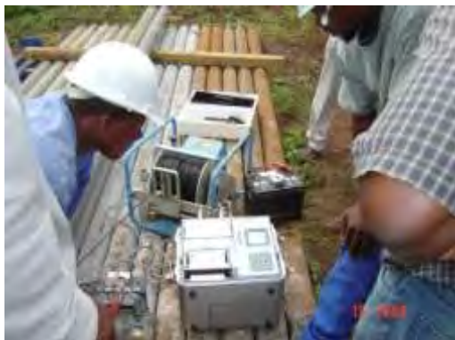
11. Explaining operation and measurement with Geologger
