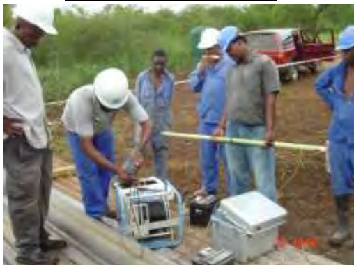
9. Connecting the probe to the winch
