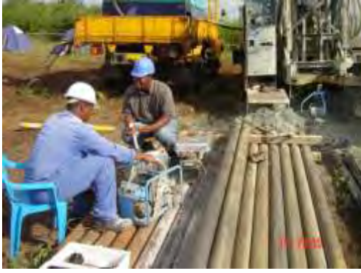
13. Trainee personnel running the borehole-logging
