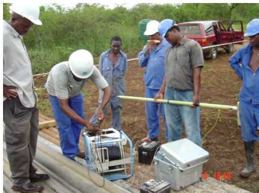
9. Connecting the probe to the winch
