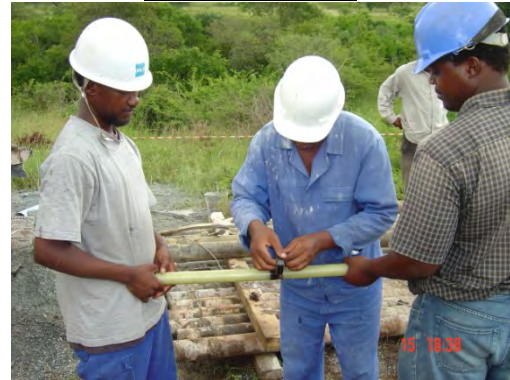
8. How to insulate the probes
