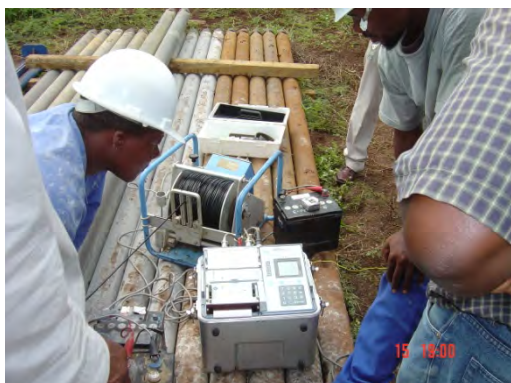
11. Explaining operation and measurement with Geologger
