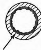
SOLIDS DEPOSITED INSIDE RODS PREVENT PASSAGE OF INNER TUBE
