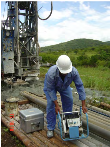
1.Measuring of the water level before Logging
