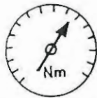
HYDRAULIC GAUGE (CALIBRATED TO SHOW TORQUE)
