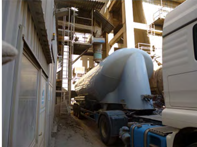
Photo 3-14 Truck for ash transportation
