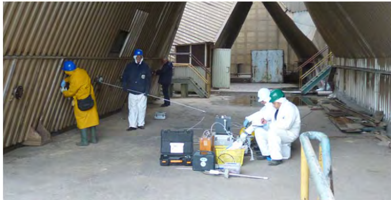
Photo 4-7 Dust measurement by C/P members at the inlet of ESP at Kosovo B-2 boiler
