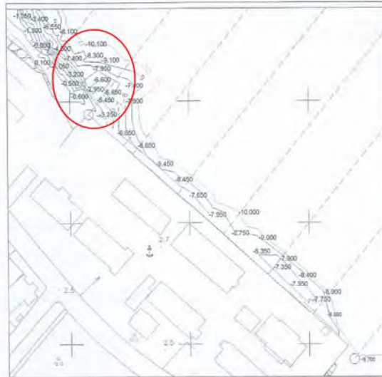
Pic.17. Detail Bathymetric map alongside quays of Dili Port at Nov 2013 made in Contractor JO around of the Wharf.
