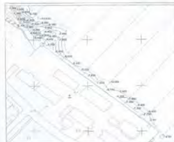
Pic.17. Detail Bathymetric map alongside quays of Dili Port at Nov 2013 made in Contractor JO around of the Wharf.
