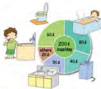
Figure 8 Daily amount of domestic wastewater
