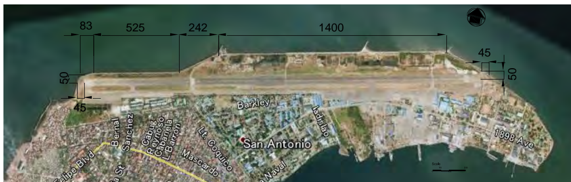
Figure 9.1.2-3 Layout of Existing Revetment
