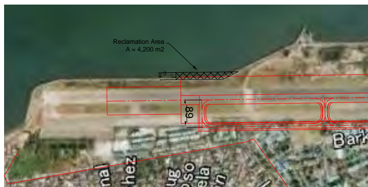
Figure 9.4.2-2 Reclamation Area in case of Threshold Offset by 330 m to RWY07
