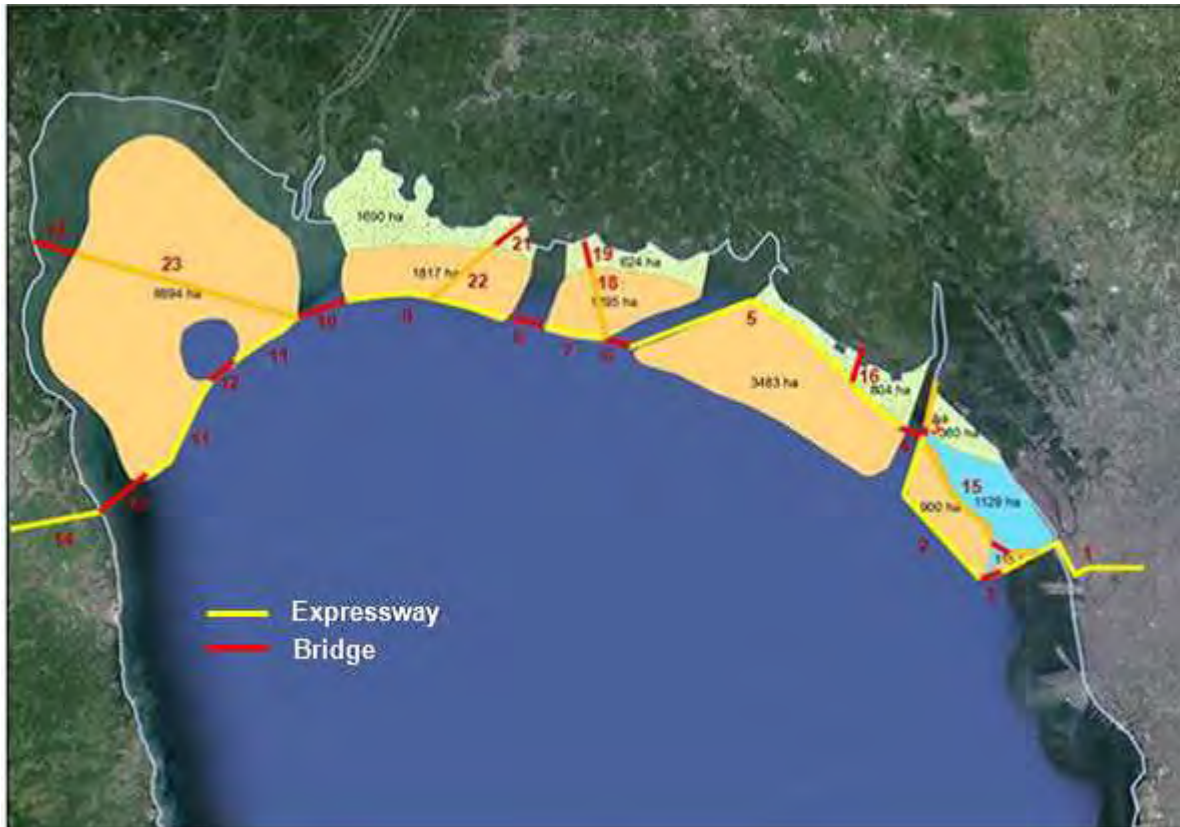
Figure 6.2-13 Manila Bay Integrated Flood Control, Coastal Defense and Expressway Project (Source: DPWH)
