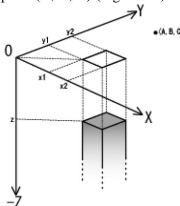
Fig. 3-2.98 Conceptual diagram of three-dimensional gravity inversion of basement relief
