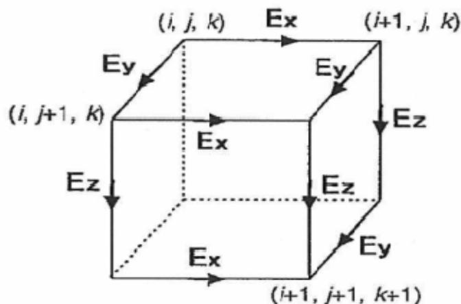
Fig. 3-2.65 Conceptual illustration for Staggered Grid configuration (After Sasaki, Y., 1999)
