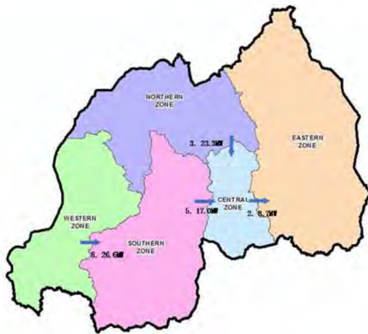
Fig. 2-5.7 Load Flow System in 2014 (Wet Season)
