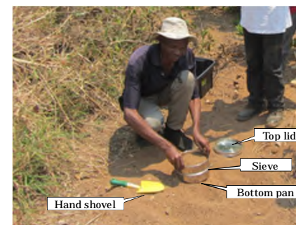
Photograph-14 Loading sediments into stainless steel sieve set
