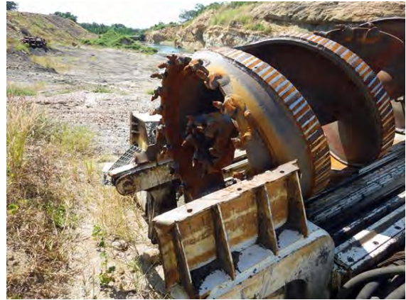
8 : Drill bit of auger
