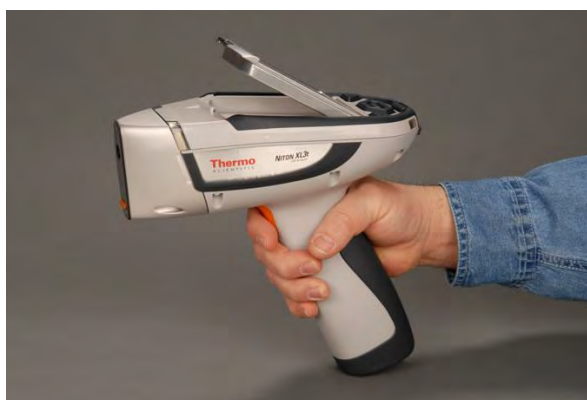
Portable XRF Analyser : Niton XL3T (from WEB site of Thermo Scientific)
