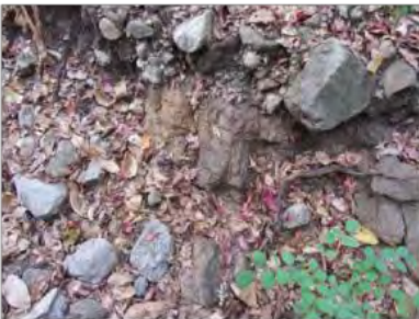
KT39: Magnetite-rutile-garnet bearing sediments. Limonite-hematite gossan with bornite stain. Highly weathered Bt gneiss-Qz vein (partly graphite gneiss). [Cu: 36.4ppm, Co: 25.3ppm, Cr: 154ppm, Ni: 94.6ppm]
