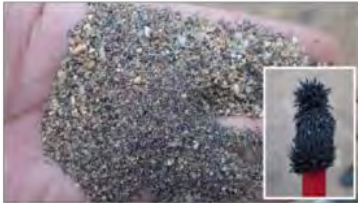
HM42: Heavy weathered magnetite-bearing Bt-Hb-gneiss with siliceous layer. [Mo:8.73ppm, Zn:203ppm, W:4.1ppm]
