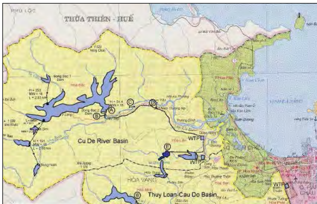
Figure 4.4 Locations of Water Supply Options suggested in the ADB Report (Location D has selected as a raw water intake point in the PS. Please see evaluation of each candidate site in “5.3 Raw water intake facility”)
