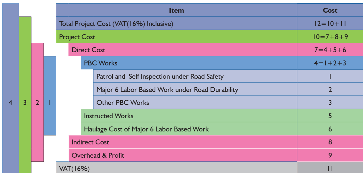
Figure I-2 Cost Estimation Structure under COSTES for PBC 2015
