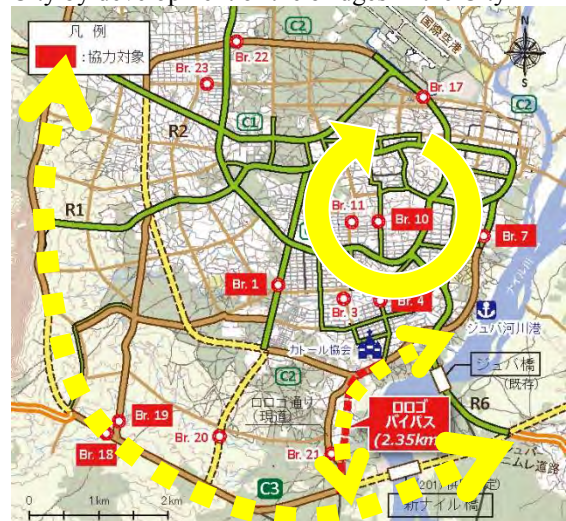
Step-3: Development of international logistics road by erection of bridges located on Ring Road C3
