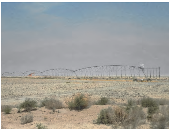
Al Okaily WUA: Photo shows pivot type sprinkler installed using subsidy system of MoA. Water is directly diverted from the Tigris river. (Basrah District)
