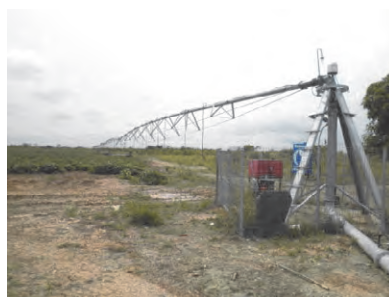
Large scale sprinkler (Center pivot/ linear type)
