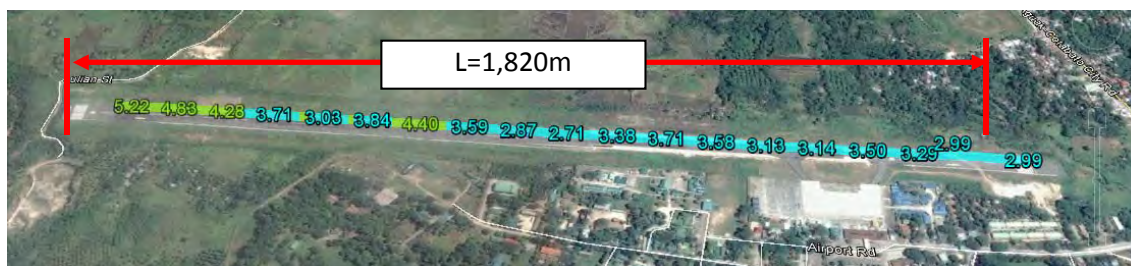
Figure 2-15.2 Example of Calibration Result at Runway of Cotabato Airport
