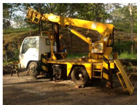
Boom truck owned by LASURECO (with missing bucket at boom top)
