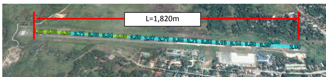
Figure 8.2 Example of Runway Calibration at Cotabato Airport
