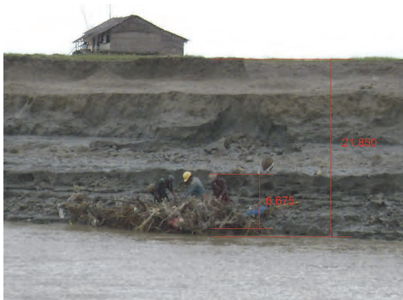
Figure 6-1: A Sample of Height Estimation by AutoCAD (Reference No. 4.2.1) (The above picture was taken during low tide, September 5, 2015)
