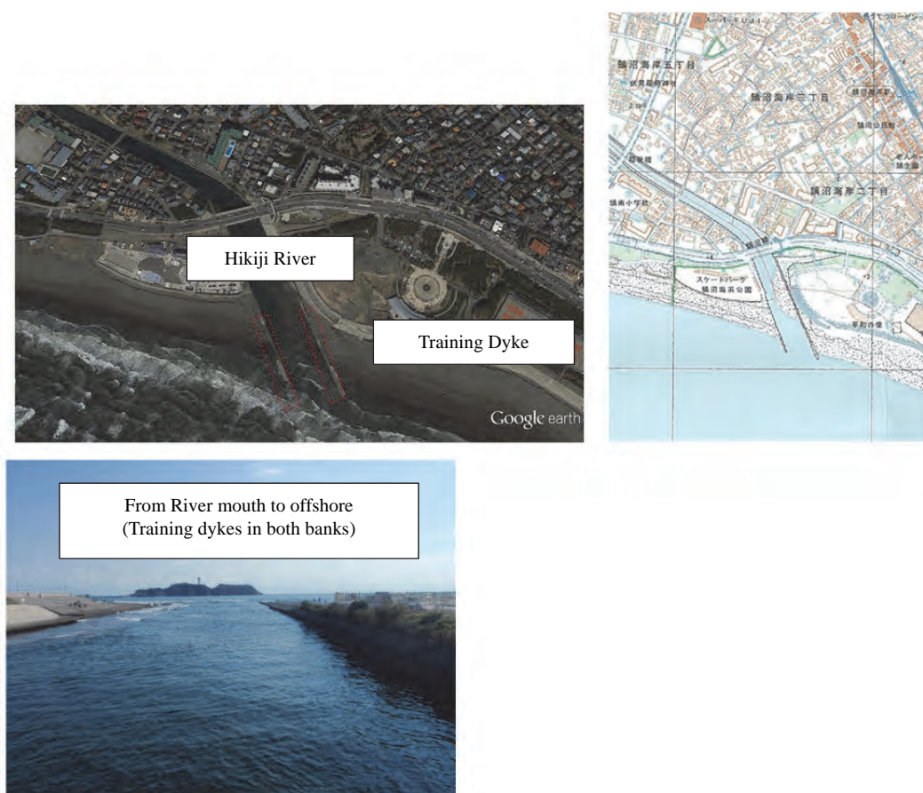
Figure A1.1. An Example of a Training Dike (the Hikiji-River in Kanagawa Prefecture, Japan)
