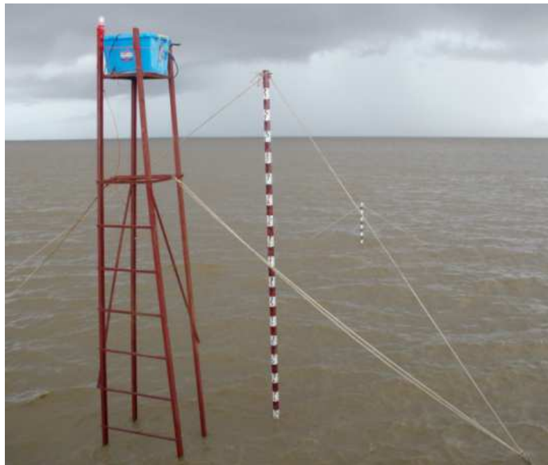
Temporarily established tide staff and automatic tide gauge at Elephant Point
