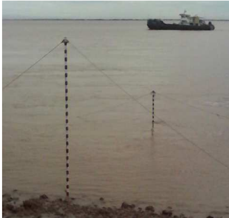
Temporarily established tide staff at Elephant Point
