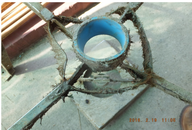
Damage Condition of steel frame and Sensor of Wave Observation
