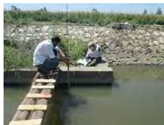
Discharge Measurement at Karadwah Canal
