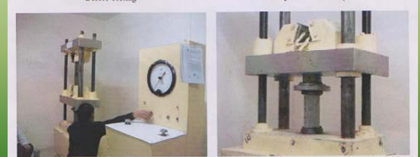
Compressive Strength Test of Concrete Cylinder
