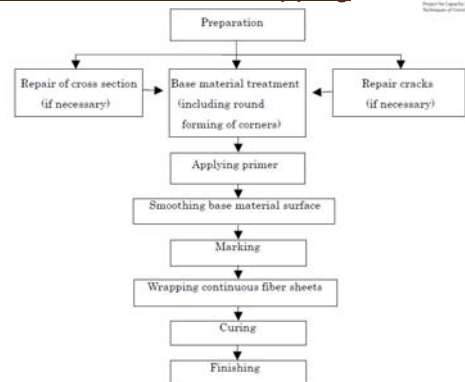
Figure 4.9-1 Flow of standard construction procedure
