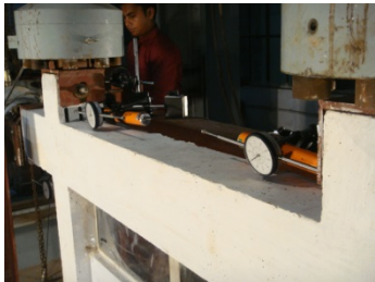
Setting of Displacement transducer and Dial gauge
