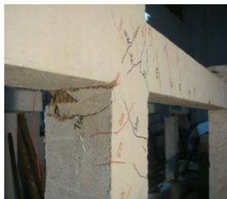
Flexural crack on beam, shear crack at panel area
