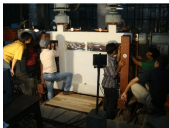
Setting of Displacement Transducer and Dial Gauge
