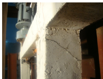
R=1/50, 6 th cycle, bottom of left column
