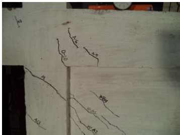
Diagonal crack width of left column is 0.3mm, right column is 0.1mm shear crack of column
