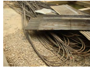
(c) Folded re-bar with 12 m length
