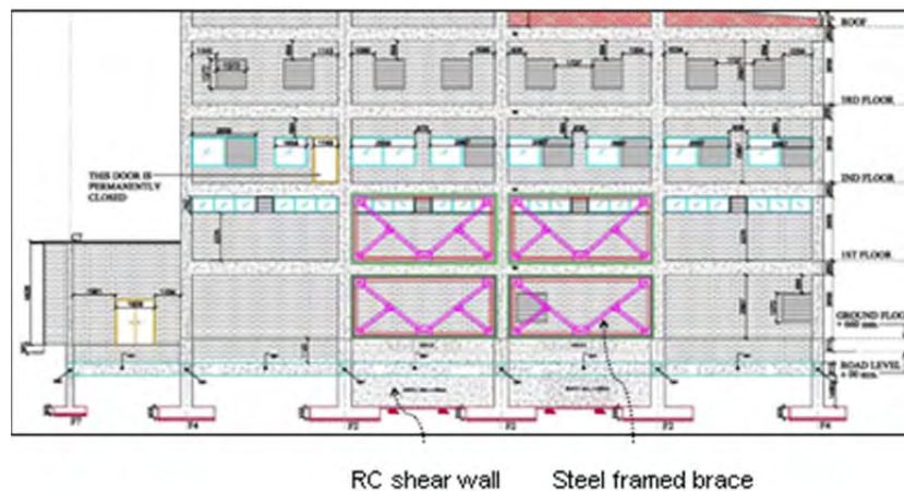
Figure 2.5.3 Framing elevation of RMG Factory 1
