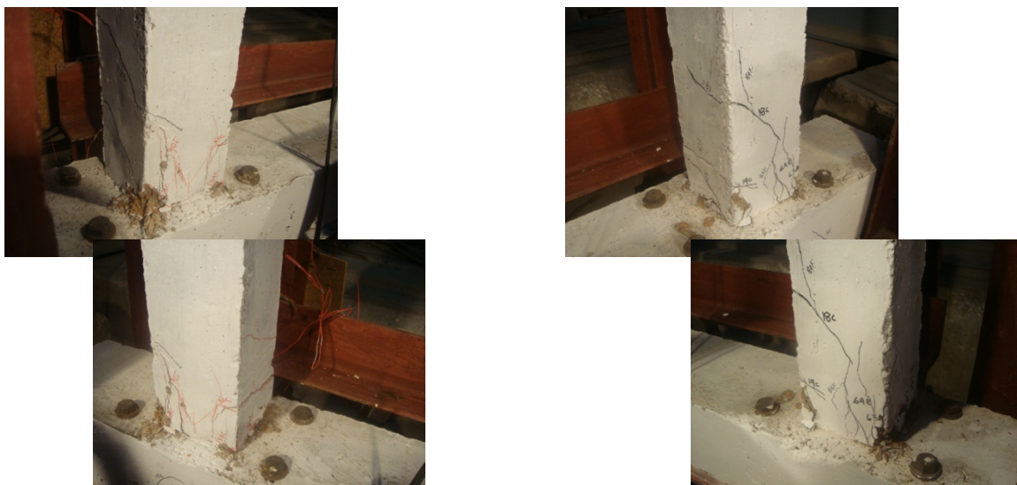
Specimen No.5, Concrete cracks and failure of covering concrete
