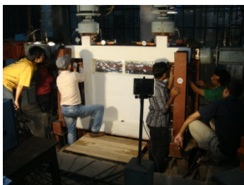
Setting of Displacement Transducer and Dial Gauge
