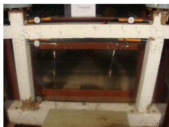
Compressive failure of covering concrete
