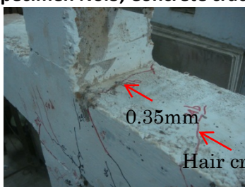
Specimen No.5, Concrete cracks and failure of covering concrete
