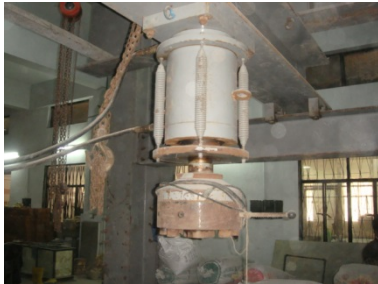
Hydraulic jack and load cell (1)
