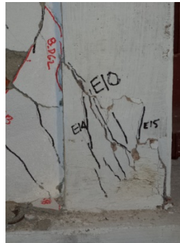
Shear failure of right column (front and rear side)
