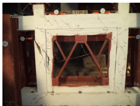
Failure at deflection 20.9mm
