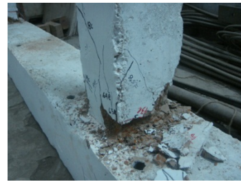
Left column, flexural crack 1.0mm Right column, flexural crack 0.25mm and compressive failure
