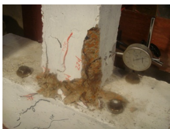
R=1/50, 6 th cycle, bottom of left column
