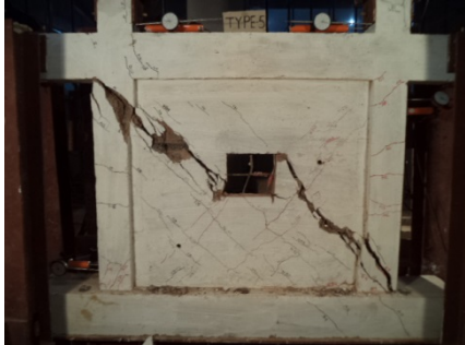
Failure n at deflectio 38.5mm
