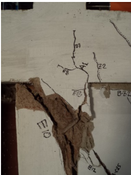
Shear failure of left column
