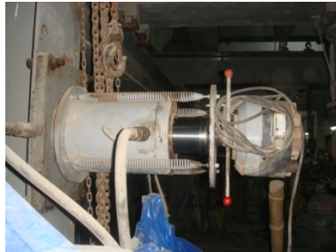
Hydraulic jack and load cell (2)
