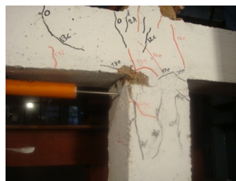
shear crack, width 1.2mm
