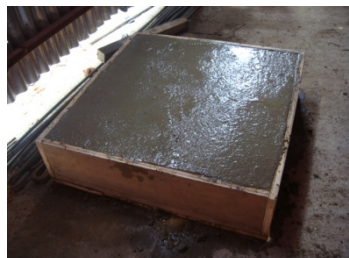
Plain concrete for core sampling
