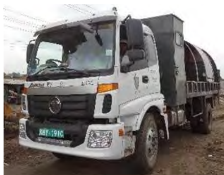
Photo 2-14 Side Loader (7-ton capacity)
