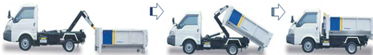
Figure 2-10 Loading a Rectangular Container with an Arm Roll Truck
