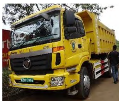
Photo 2-15 Tippers (14-ton capacity)
