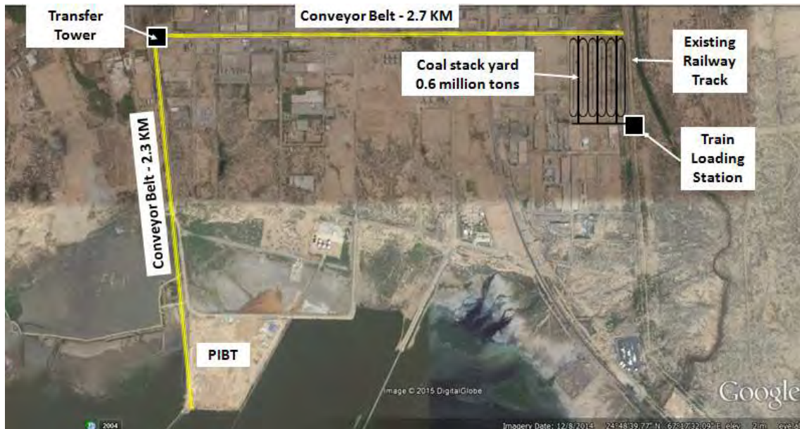
Figure 3.5 Concept Development Routes Plan of Coal Transport by Belt Conveyors
